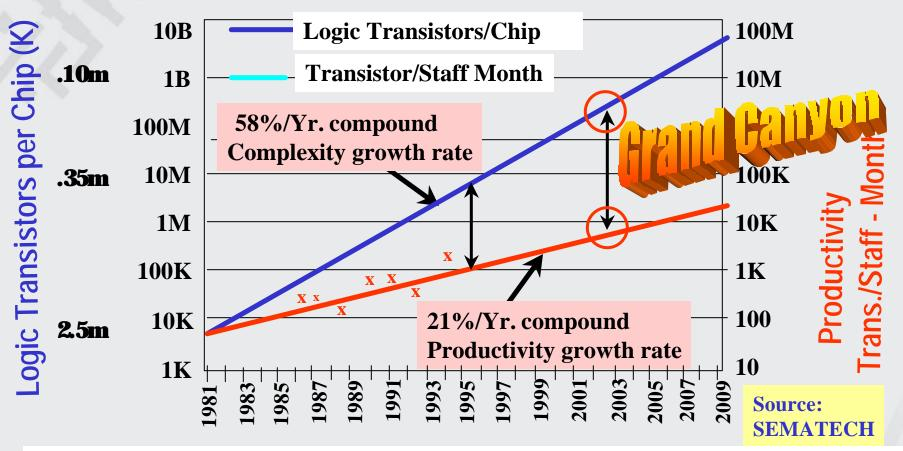
100M logic gates in 90nm = Logic of 1000 ARM7's
