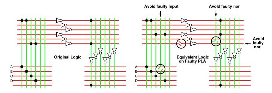
All components (PLA, routing, memory) interchangeable; Have M-choose-N property Allows local programming around faults
