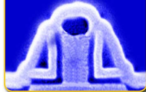
65-nm Transistor Cross Section
