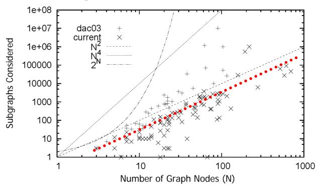
Number of subgraphs considered using an output port constraint of two
