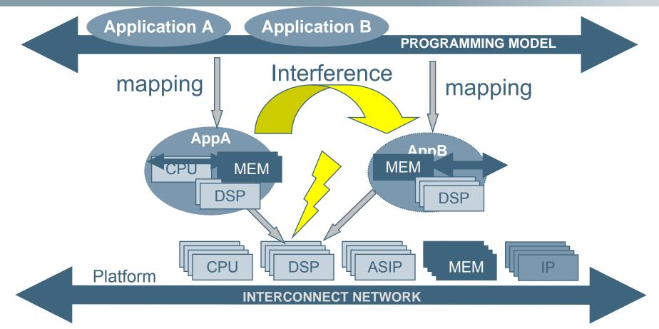
**Design-Time Mapping Predictability**: how to ensure that multiple independently mapped applications will simultaneously work with the same behavior on a single platform
