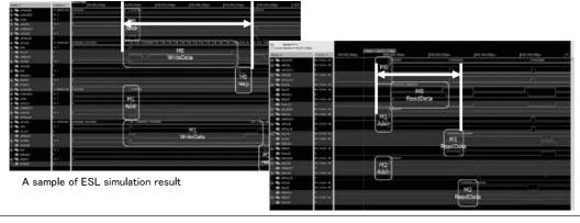
The bus collision has been happened also between independent threads of neighbor CPU
