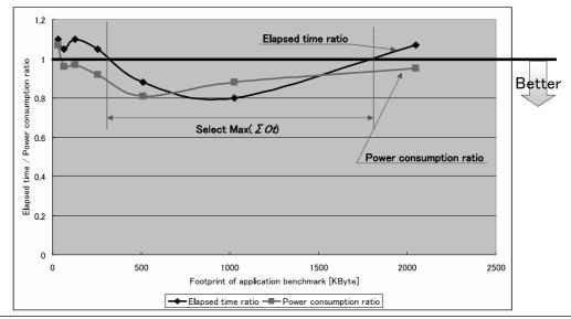
The figure is dividing of the elapsed time and the power consumption of the proposal scheme by the result of original scheme.
