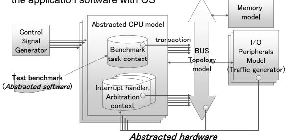
The abstracted modeling is effective to know the characteristic of object hardware. And also the software that operate many threads should be abstracted to simplify the system.
