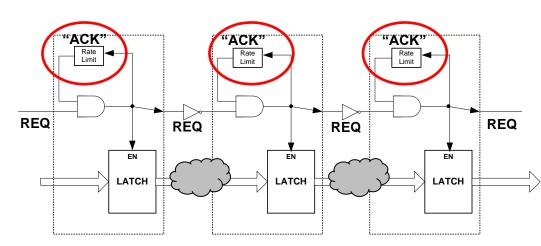
Octasic has modified the approach - no ACK but a rate limiter:
