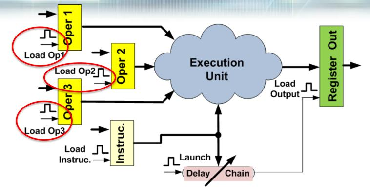
• The operand state registers are asynchronously loaded
