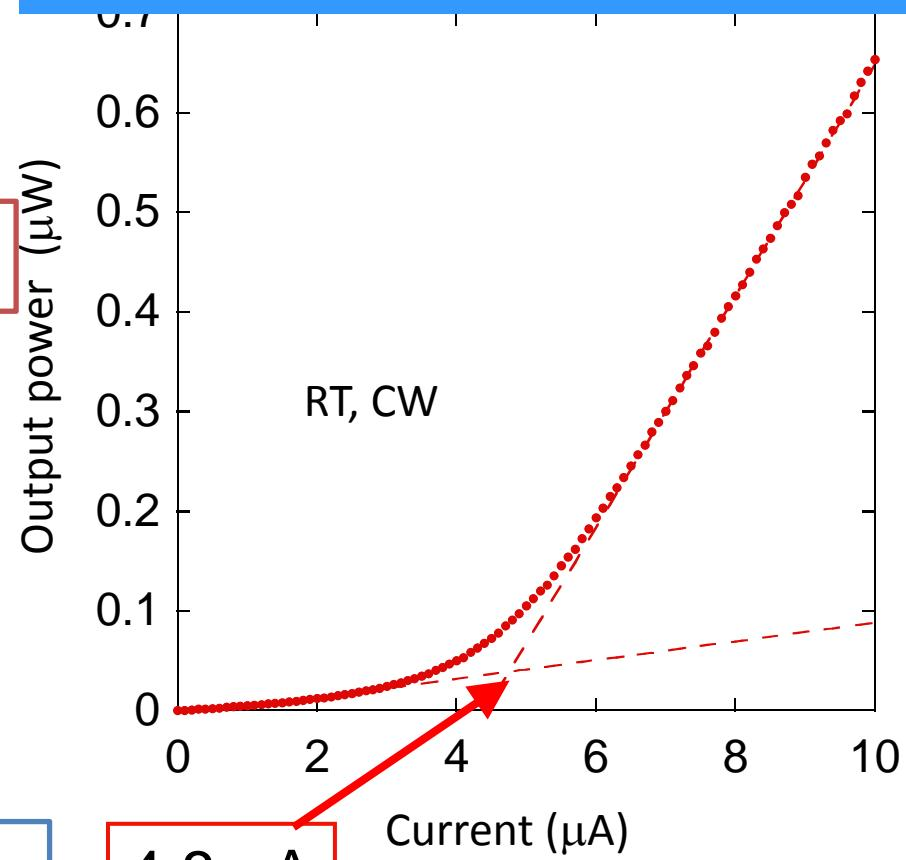
**World's lowest threshold for any type of laser diode**
