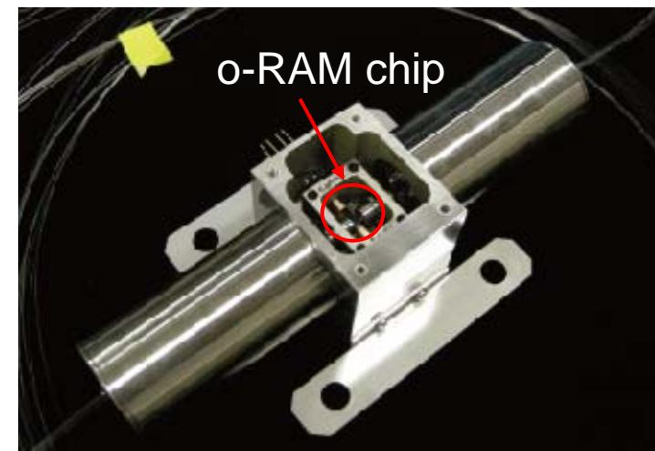
Fiber module equipped with o-RAM chip used for experiment
