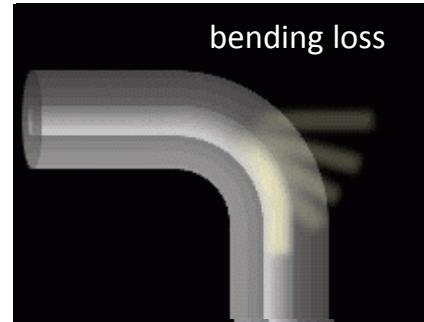
Leakage at bending
