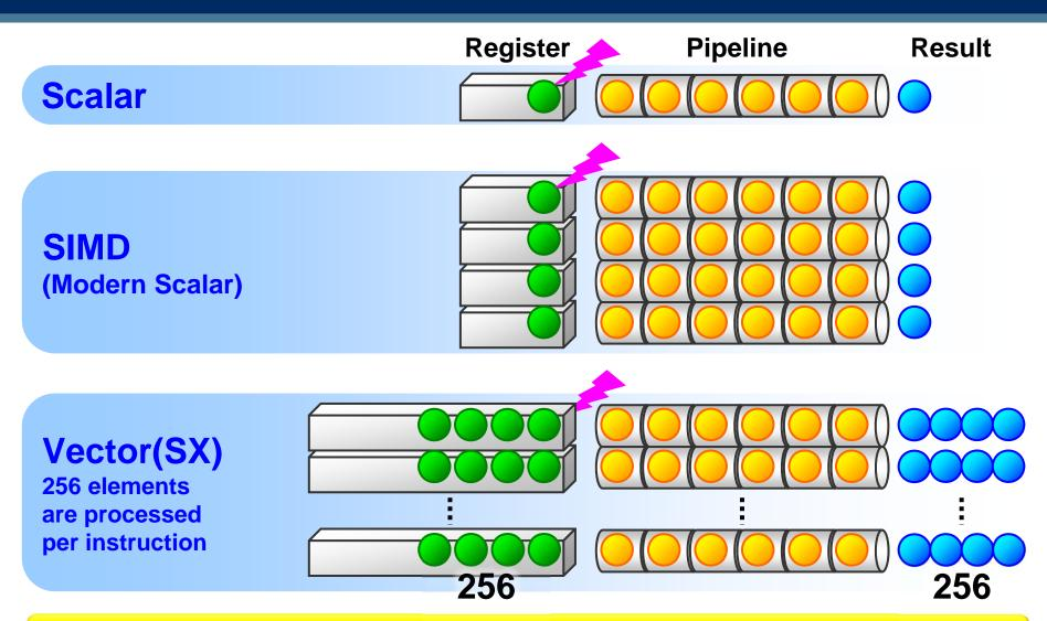
Vector is efficient to fill pipelines and to hide latencies
