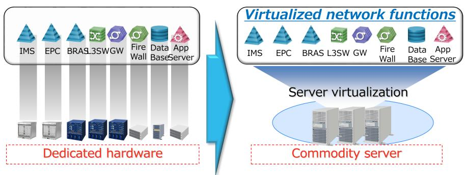
IMS,EPC: network equipment used in mobile core network BRAS: network equipment used in fixed access network
