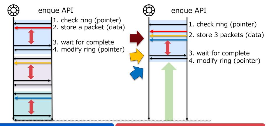
One by one packet transfer is inefficient Multiple packets transfer improves performance
