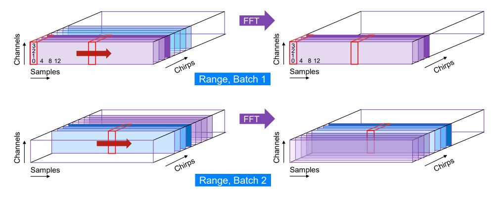
While FFT processes data using one set of buffers, DMA transfers fill/empty another set of buffers
