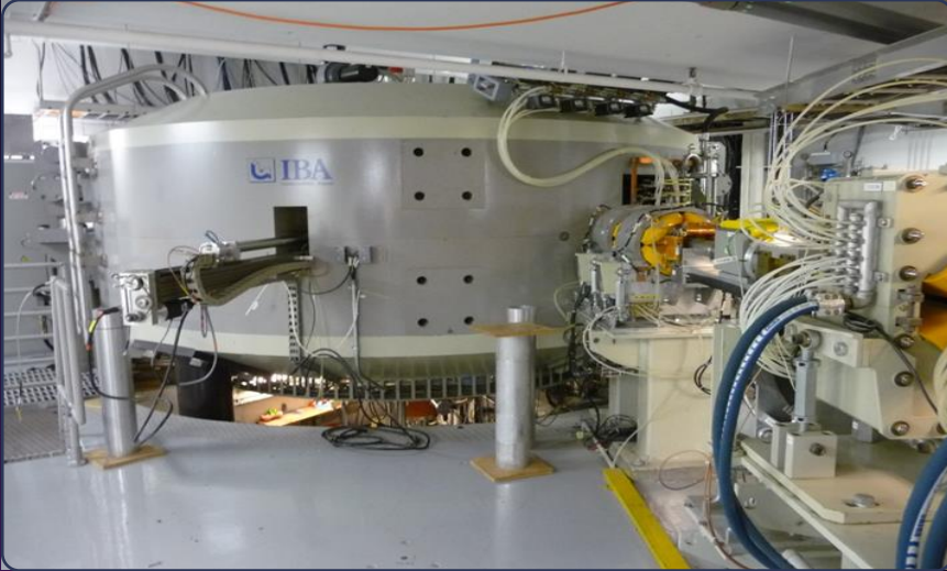
Ground: accelerator / proton-beam irradiation — SEE screening & coverage measurement
