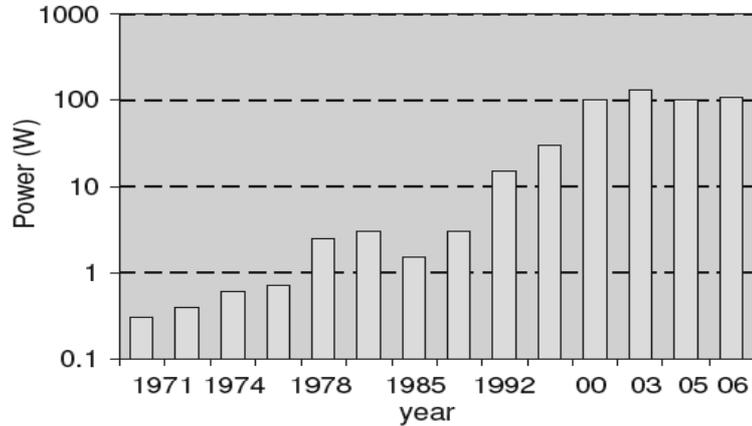
Power consumption of Intel microprocessors from 1970 to 2006
